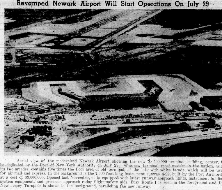
Aerial view of the modernized Newark Airport showing the new $8,500,000 terminal building, center, to be dedicated by the Port of New York Authority on July 29. The new terminal, most modern in the nation, with its two arcades, contains five times the floor area of old terminal, at the left with white facade, which will be used for air mail and express. In the background is the 7,000-foot-long instrument runway 4-22, built by the Port Authority at a cost of $9,000,000. Opened last November, it is equipped with latest runway approach lights, instrument landing system equipment, and precision approach radar flight sight aids. Busy Route 1 is seen in the foreground and the New Jersey Turnpike is shown in the background, paralleling the new runway.
